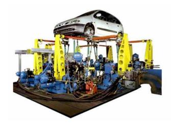
The vibration environment is incomplete without rotation. The MEMA Type 6 DOF Shaker Tables are available for these types of testing. The arrangement of shakers among all three axes allows the roll, pitch, and yaw to be achieved along with the three-dimensional translation motions from the table.
