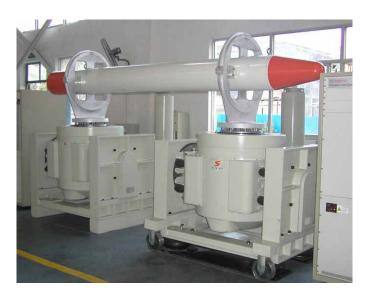
Three axis shaker tables are available for Multiple-Exciter Multiple-Axis (MEMA) test arrangements. Many testing applications require testing the DUT simultaneously in all three directions. With a three- axis shaker table system, the overall testing time is reduced by two-thirds in comparison to single-axis testing along each axis. More importantly, it identifies failures otherwise undetected with single-axis testing.
