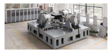
Crystal Instruments' Spider MIMO Control System takes use of multiple shakers and assigns multiple control channels with defined profiles. The control process of MIMO Control is expanded into a Matrix fashion, unlike the Scalar fashion of single shaker control.
