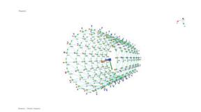
During the majority of time, the structure under test is more complex than a simple plate. The Geometry feature of the Modal software will process this type of structure under testing using Components. Each component has its own origin and defined Euler angle. This allows the component to take use of its own local Cartesian coordinate system for directions.
